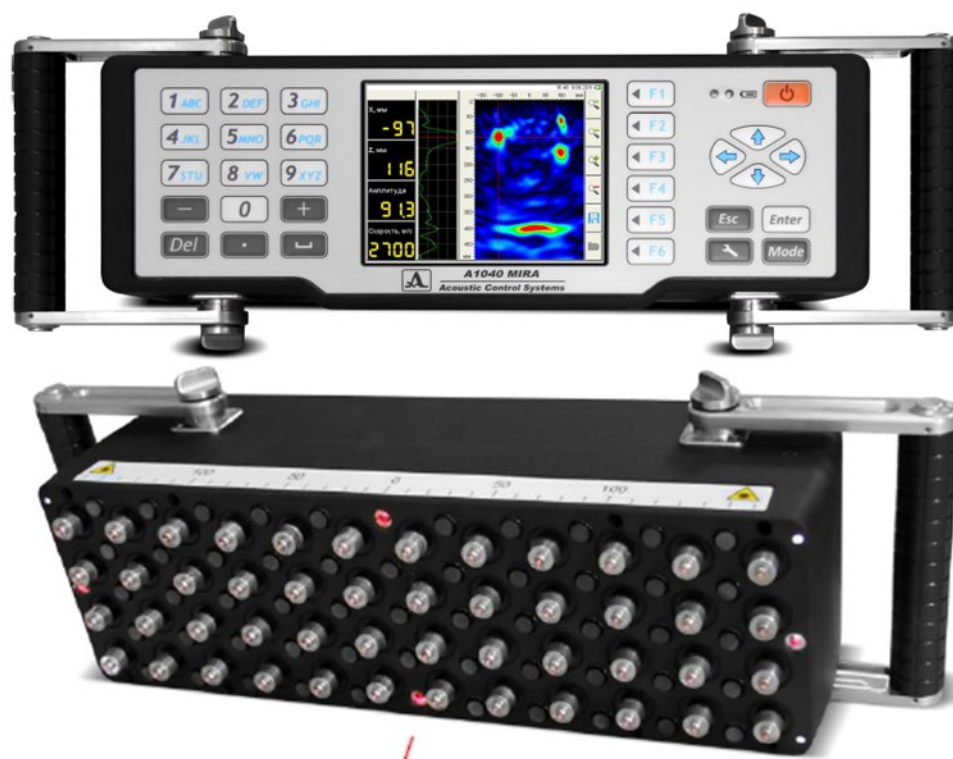
Figure 2-10 MIRA device (Acoustic Control Systems 2015)
